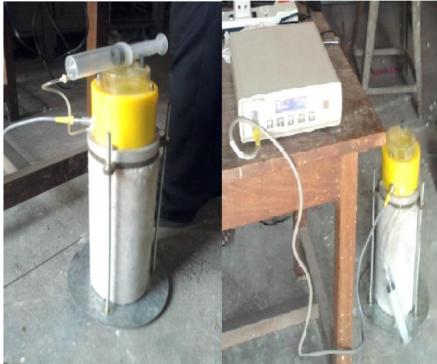
Fig 3 permeability tests on cylinder specimen
